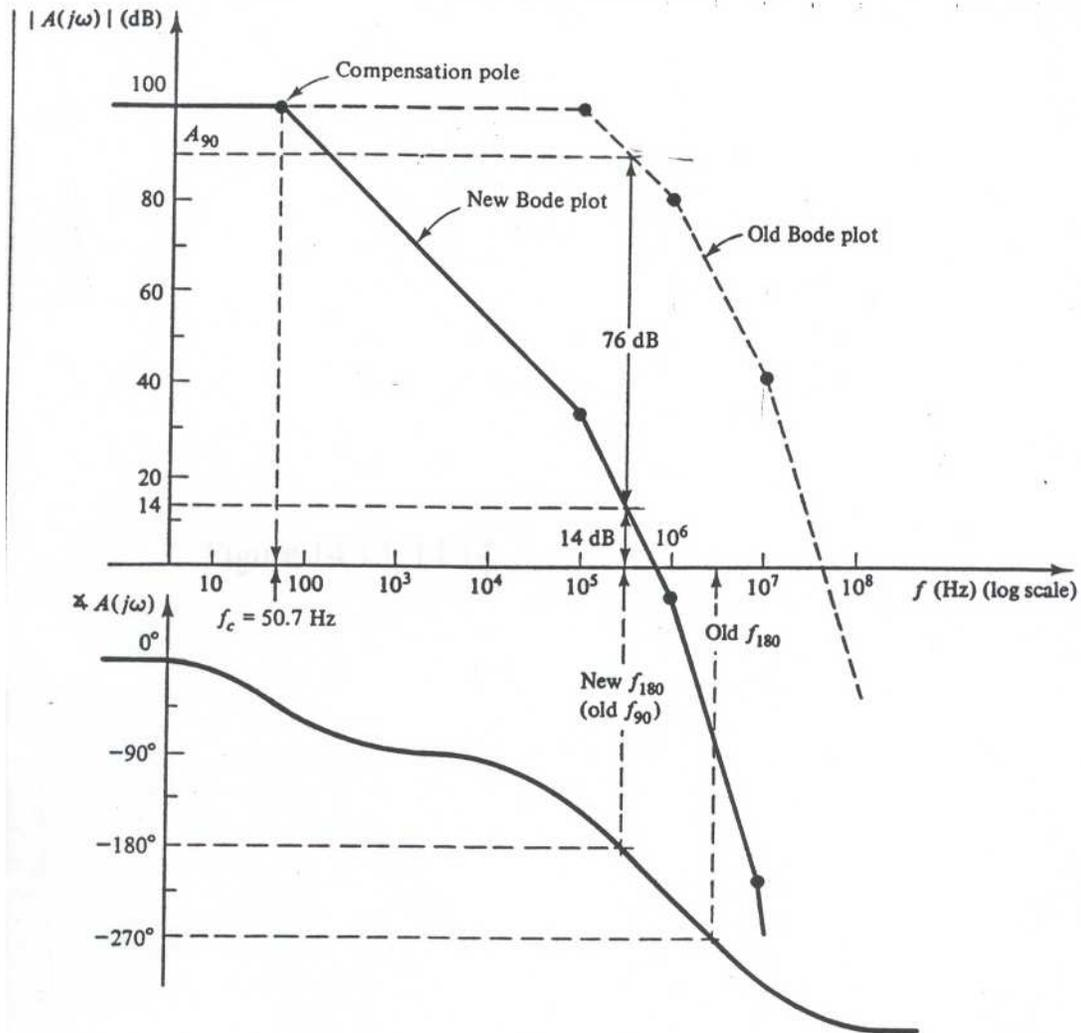
Figure 14.13 Bode plot of the op-amp of Fig. 14.12 minimally compensated for  $\beta = 1/5$  by the addition of a dominant pole at  $f_c = 50.7$  Hz. The gain is reduced to +14 dB at the old  $f_{90}$ . The old  $f_{90}$  becomes the new  $f_{180}$ .
