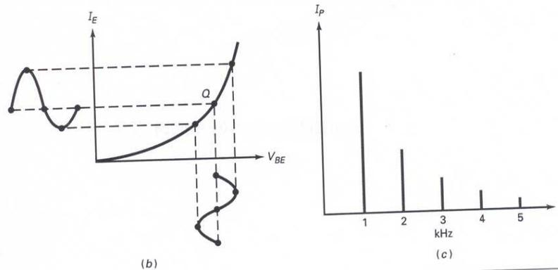
The degree of harmonic distortion is measured by the percent of total harmonic distortion, THD, and defined as:
