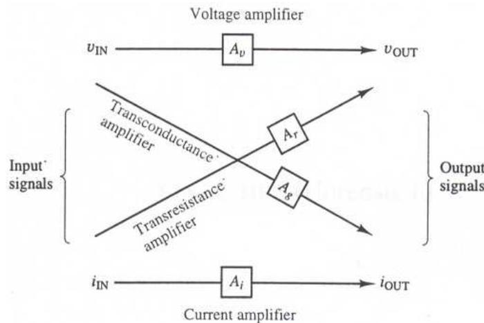
a. A *voltage amplifier* with gain  $A_v$  accepts a voltage as its input signal and provides a voltage as its output signal.
