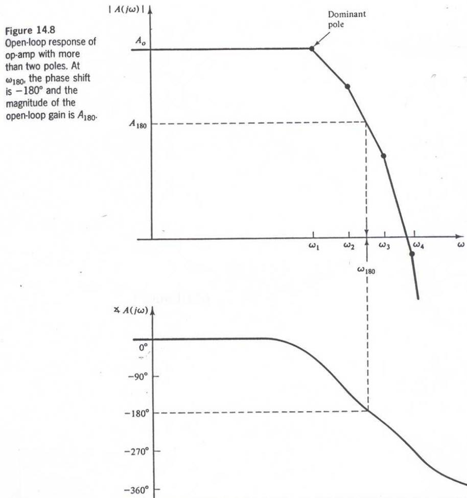
At some frequency,  $\omega_{180}$ , the  $-180^\circ$  phase shift will change an otherwise negative feedback loop into a positive feedback loop as shown below.
