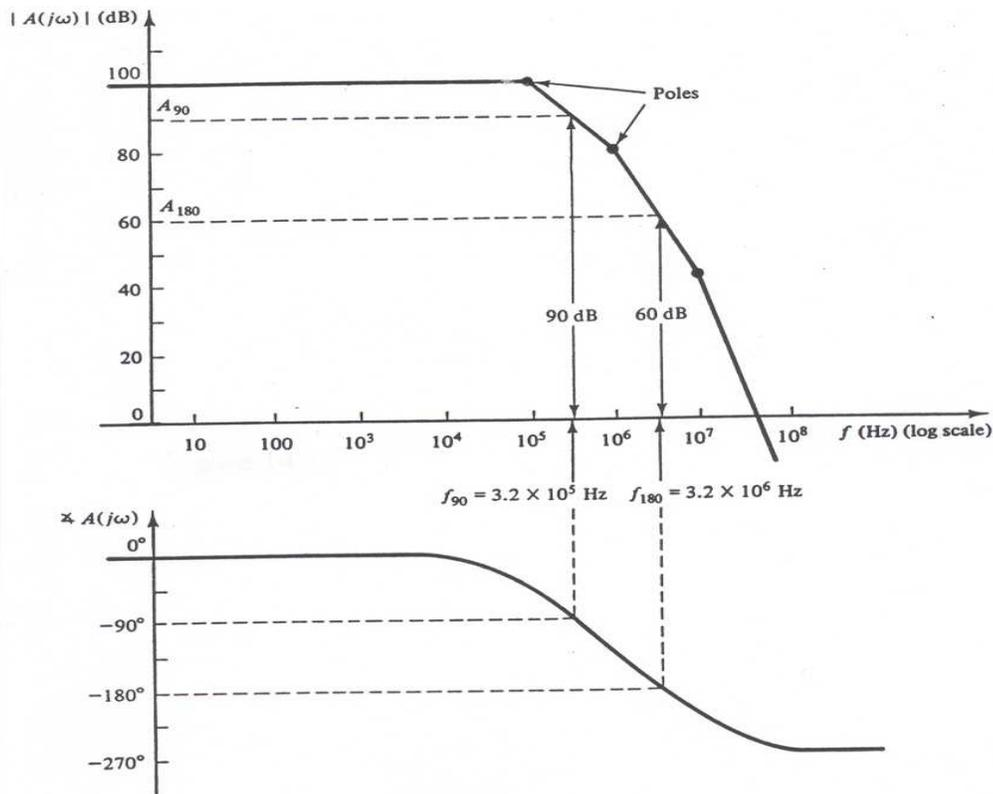
Figure 14.12 Measured Bode plot of an uncompensated op-amp. The gain is equal to +60 dB at  $f_{180}$ .
