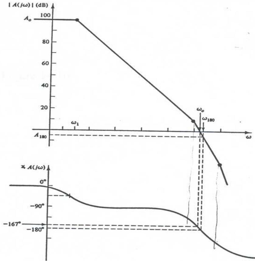
If an op-amp is not internal compensated for all feedback conditions, its feedback loop must be evaluated for stability. If the feedback loop is unstable, external compensation must be added. External compensation is sometimes preferred over internal compensation because the latter limits the gain bandwidth product of the feedback loop.
