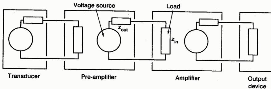
Figure 1: An instrumentation system is a chain of voltage source and load
