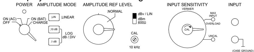
The UNCAL indicator light found to the right of the INPUT SENSITIVITY knob will light when the CAL adjust knob is not rotated fully clockwise. This means that the display of the analyzer is uncalibrated, and therefore inaccurate. Always rotate the CAL knob fully clockwise so that the UNCAL indicator stays off.
