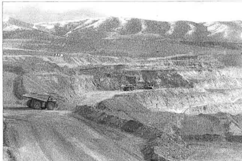
Figure 9: Photo of the upper northeast wall of the Betze-Post open pit showing the location of crest offloading in the Midnight/Pats complex wedge.
